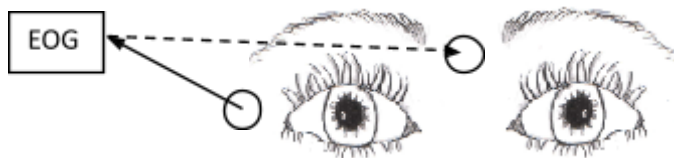
Figure 4. EOG electrode placement - combined vertical and lateral eye movement
