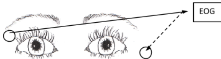
Figure 4. EOG electrode placement - combined vertical and lateral eye movement
